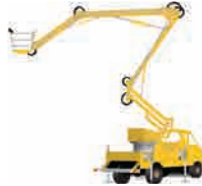
Mobile Elevating Work Platform (MEWP)
