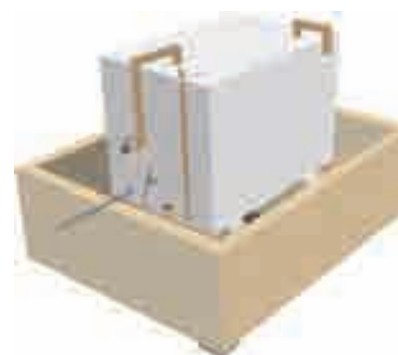
A bunded tank
