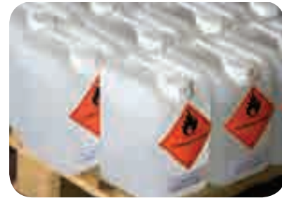
Flammable liquids must be kept in closed containers when not in use
