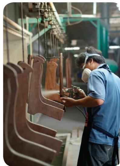
Spray-painting furniture parts with a flammable varnish at an assembly line
