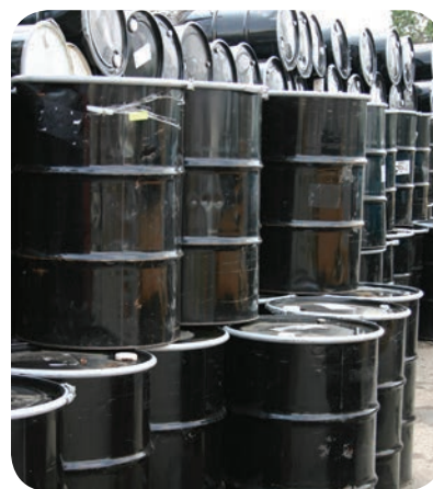
Inadequate drum storage
