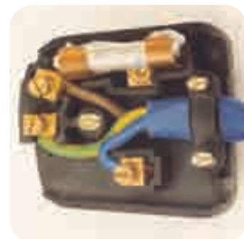
Fuse in a plug (Adapted from original source HSG107 Maintaining portable and transportable electrical equipment (2nd ed.), HSE, 2004)
