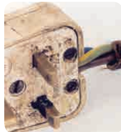
Badly damaged plug and cable Source: HSG 107 Maintaining portable and transportable electrical equipment (2nd ed.), HSE, 2004
