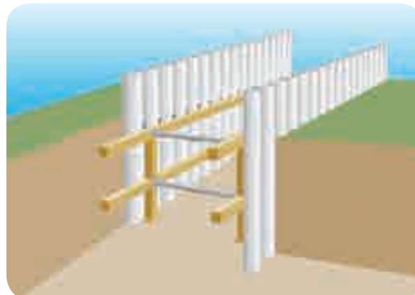
Shoring the sides of an excavation by 'close sheeting'
