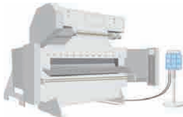
A photo-electric guard fitted to a press brake (Based on original source L22 Safe use of work equipment (4th ed.), HSE, 2014 ( www.hse.gov.uk/pubns/books/l22.htm ))
