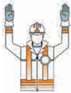
Danger (emergency stop)
