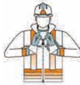
Indicating horizontal distance
