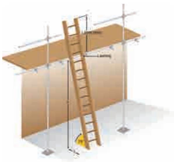
Ladder access to a working platform
