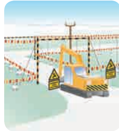
Passage of plant beneath lines (Based on original source HSG144 The safe use of vehicles on construction sites (2nd ed.), HSE, 2009 ( http://www.hse.gov.uk/pubns/priced/hsg144.pdf ))
