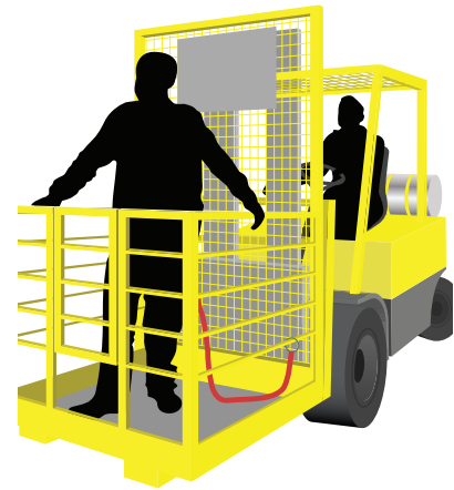
Forklift truck with non-integrated working platform
