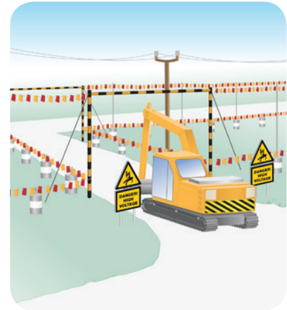
Passage of plant beneath lines (Based on original source HSG144 The safe use of vehicles on construction sites (2nd ed.), HSE, 2009 ( www.hse.gov.uk/pubns/priced/hsg144.pdf ))
