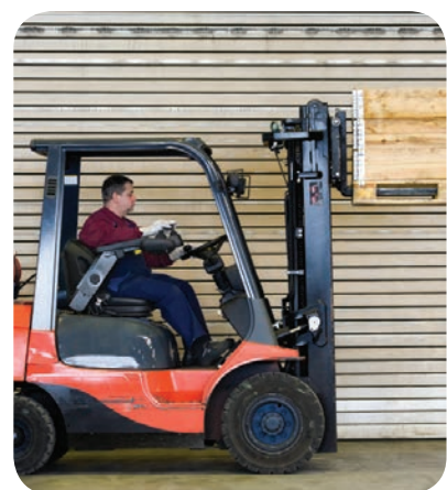
Counterbalance LPG-powered lift truck
