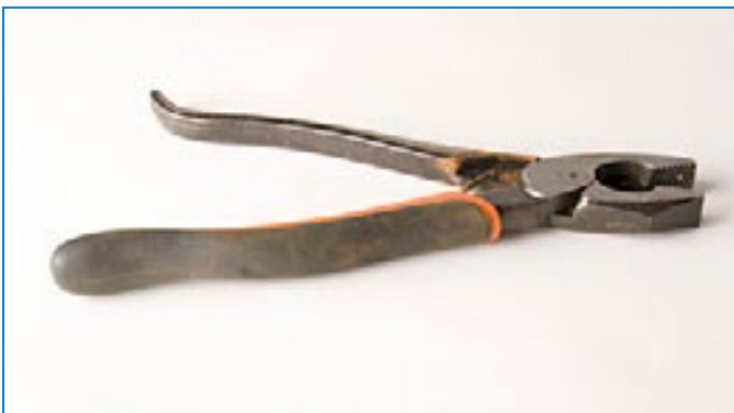
Use well-designed tools. Longer, well-contoured, wider handles spread the pressure on the hand over a larger area.
