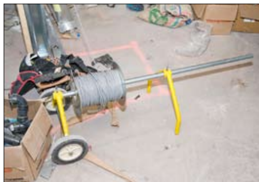
Using manual handling devices and tuggers eases the physical burden placed on workers.
