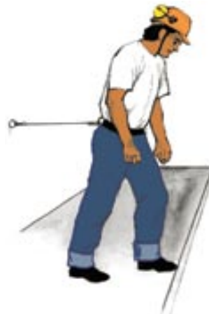
This is an example of a fall restraint system. The worker cannot fall off the edge.
