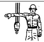
LOWER THE BOOM AND RAISE THE LOAD. With arm extended, thumb pointing down, flex fingers in and out as long as load movement is desired.
