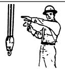
**MOVE SLOWLY.** Use one hand to give any motion signal and place other hand motionless in front of hand giving the motion signal. (Hoist slowly shown as example.)
