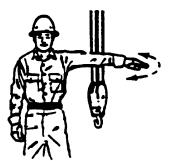
TROLLEY TRAVEL. Palm up, fingers closed, thumb pointing in direction of motion, jerk hand horizontally.
