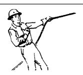
**EXTEND BOOM.** (Telescoping Booms) One Hand Signal. One fist in front of chest with thumb tapping chest.
