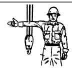
RAISE THE BOOM AND LOWER THE LOAD. With arm extended, thumb pointing up. Flex fingers in and out as long as load movement is desired.
