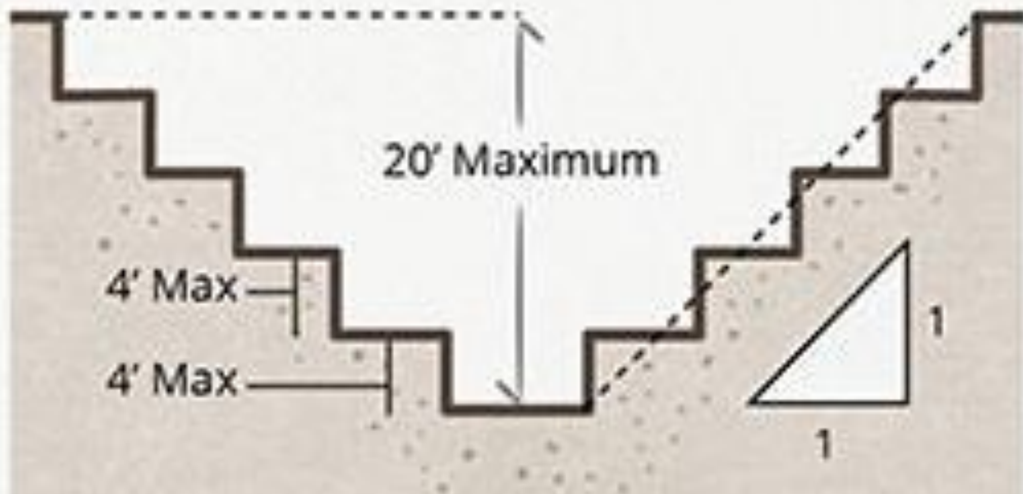
MULTIPLE BENCH EXCAVATION
